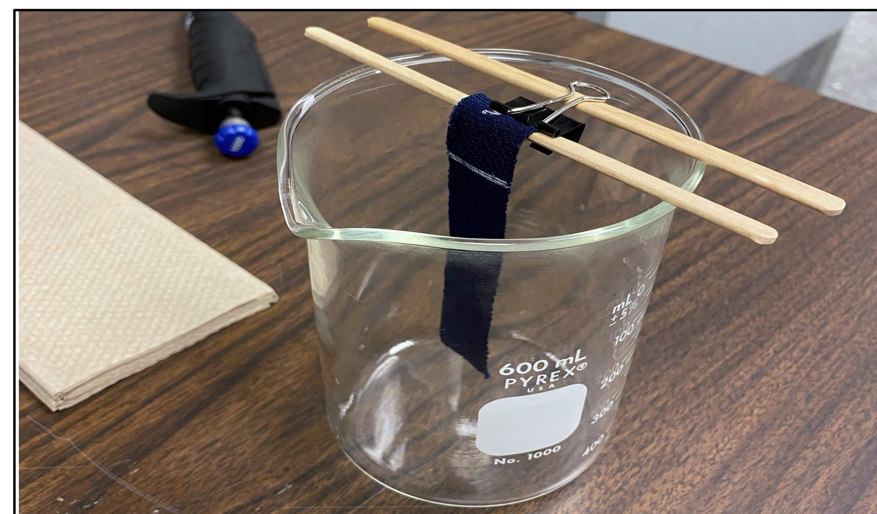
Figure 3: Vertical Wicking Test Set Up
