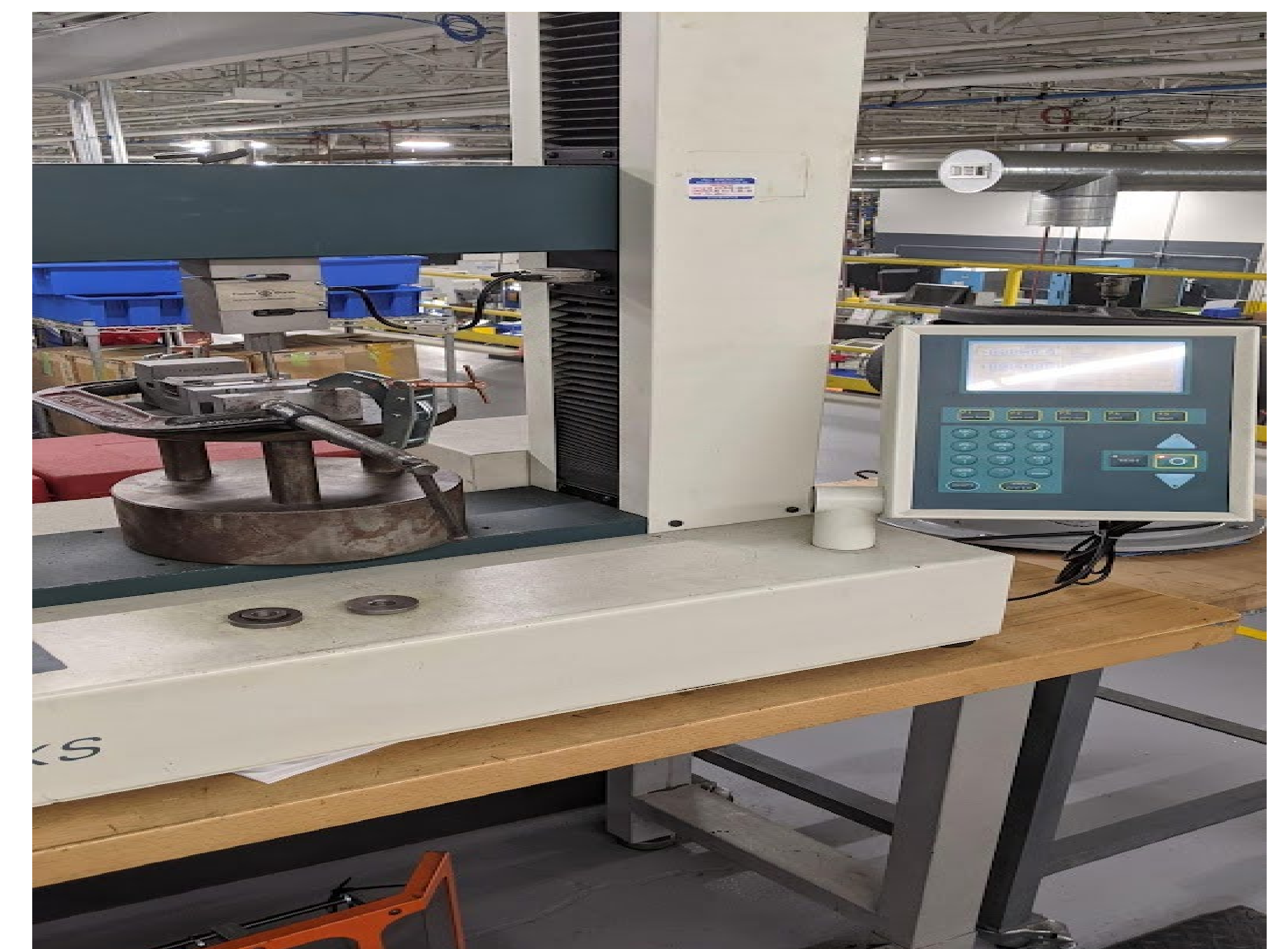
Figure 3. Testing of trigger assembly.
