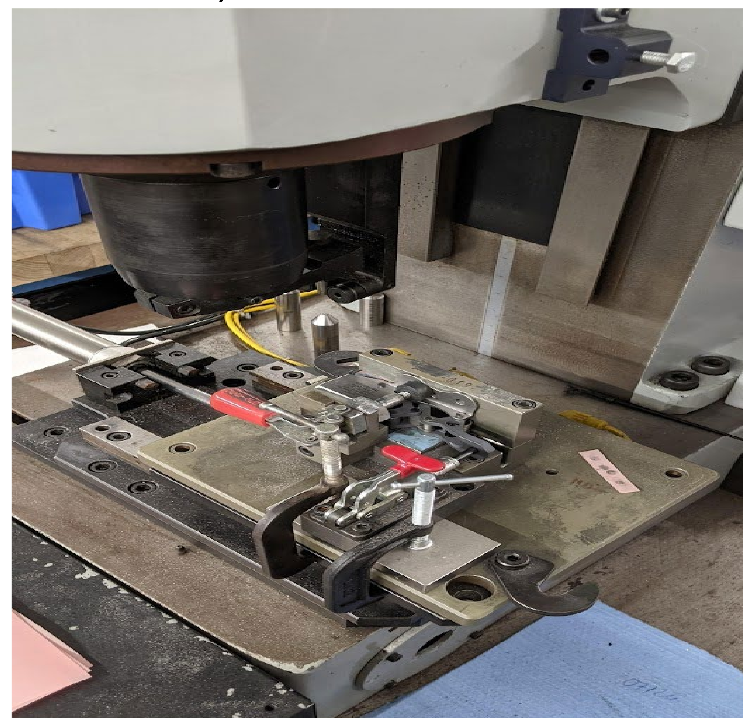
Figure 2. Redesign of riveting fixture.
