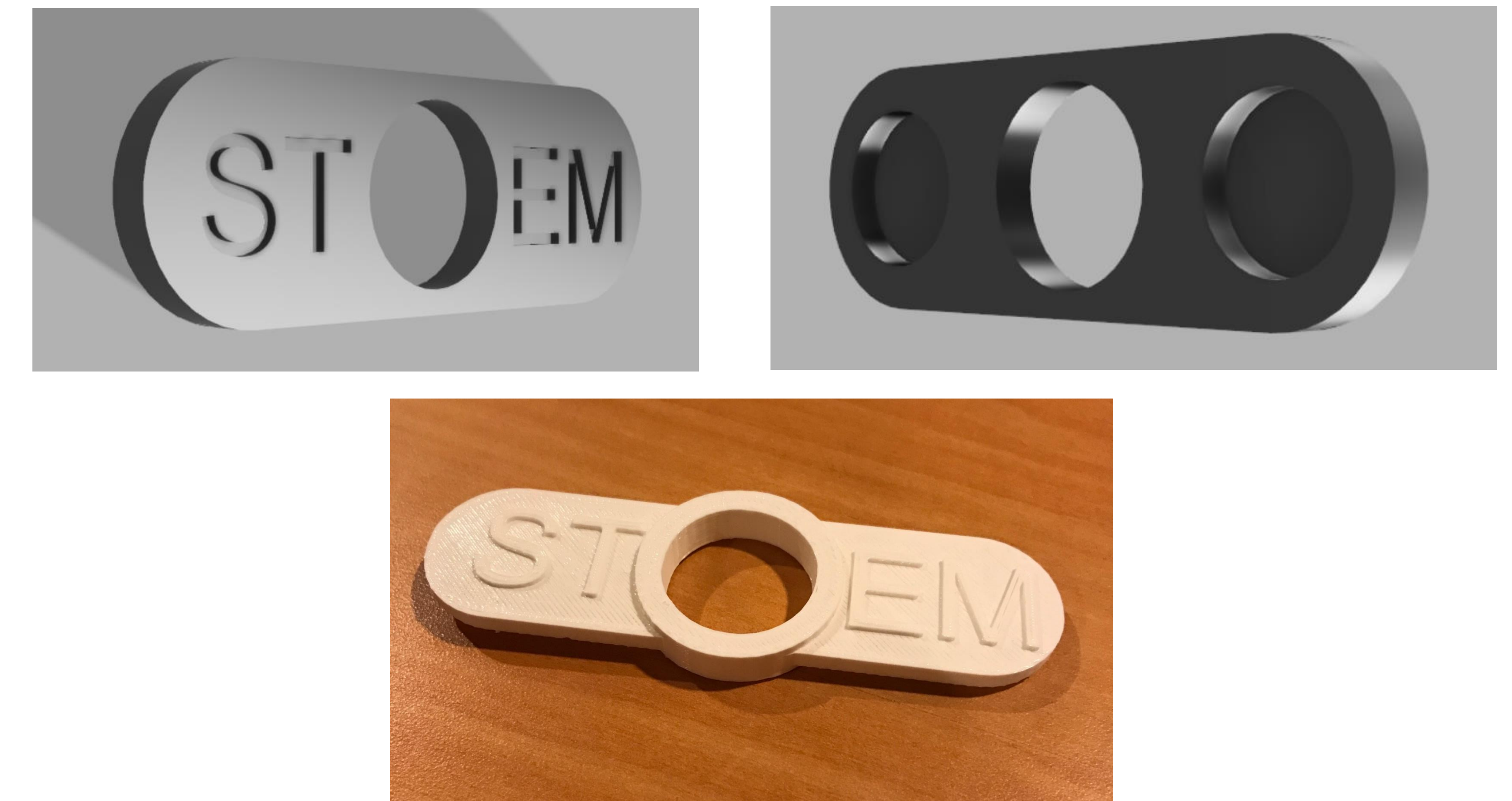
Figure 3. Spinner toy with “STEM” letters: front of spinner (top left), back of spinner (top right) which has two holes to hold two nickels each as weight, and first physical prototype (bottom).
