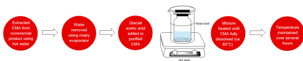
Figure 1: CMA was extracted and purified from the commercial product using hot water and rotary evaporation. Glacial acetic acid, CH 3 COOH, was added to purified commercially produced CMA. The resulting mixture was placed in a water bath and heated until CMA fully dissolved. Part of the acetic acid was then slowly evaporated off at ca. 80°C over several hours upon which large crystals suitable for single crystal diffraction formed.
