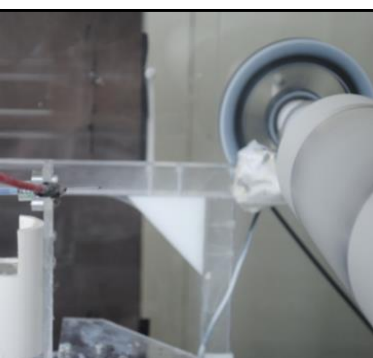
Figure 2. Electrospinning. Shows the homemade cabinet electrospinning a solution onto a mat. It uses an electrical force to thread the solution onto the collector as it spins on the rotating drum.
