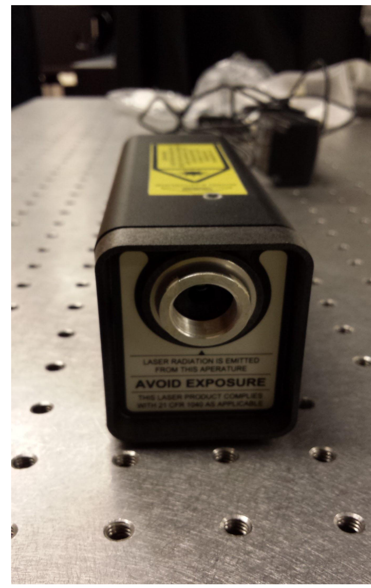
Helium Neon laser from Cleveland State University's Optics Lab
