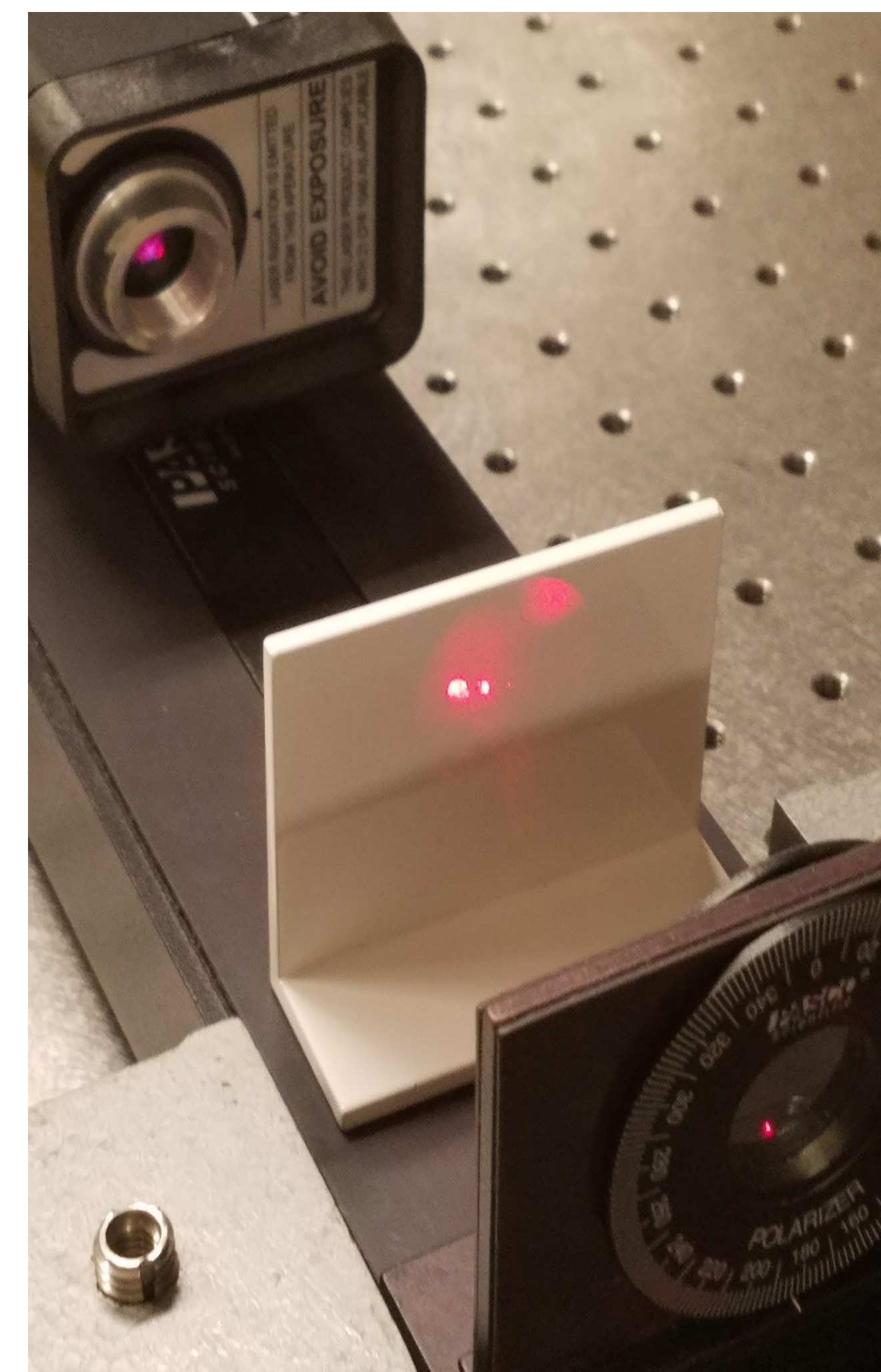
A closer look at equipment setup, featuring the Helium Neon laser and the calibrated polarizers
