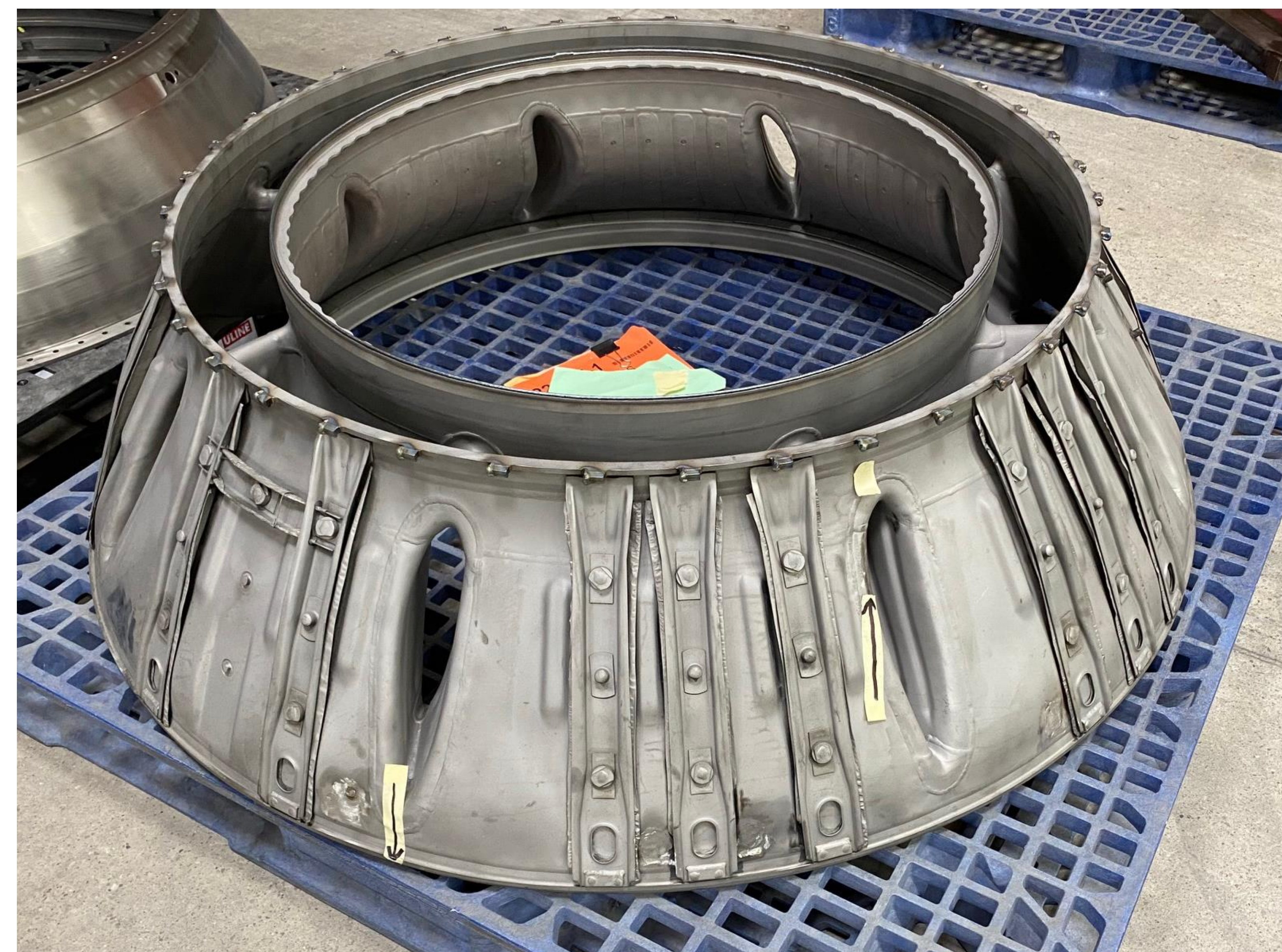
LM2500 Turbine Mid Frame, the component that I did the most work on.
