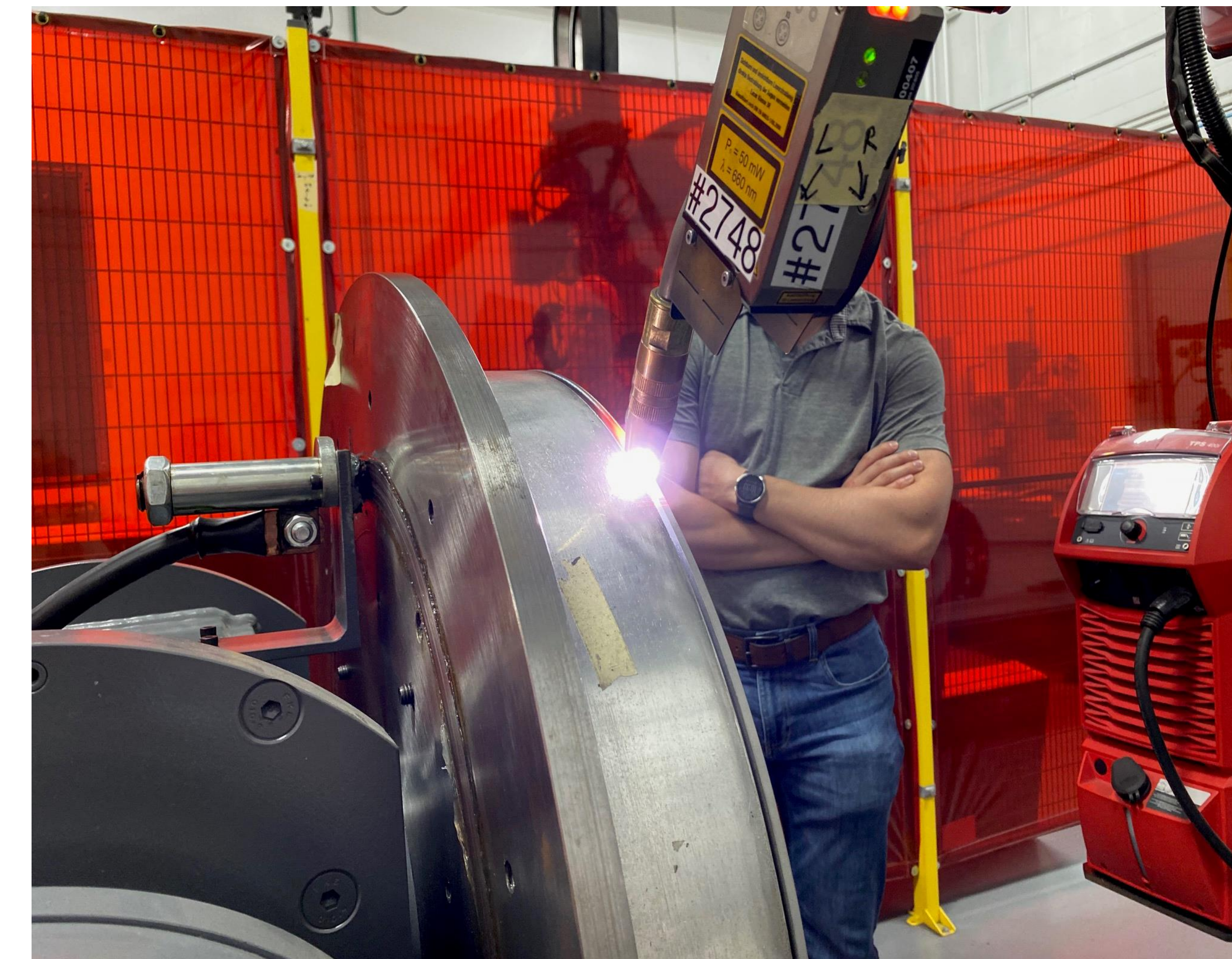
Weld test being done on a Seal Ring
