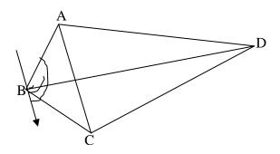
Angle measurements of B can be calculated with respect to landmark D if we know all the angles in the triangles BAC and triangle ACD. Thus the knowledge of the radial information of A and C with respect to the landmark D we get the information of their neighbor B. In the case of radial technique similar to the Euclidean method we use GPS but here we use the method of triangulation. Thus the propagation of radial information coupled with triangulation helps us to find the position of the node B.
