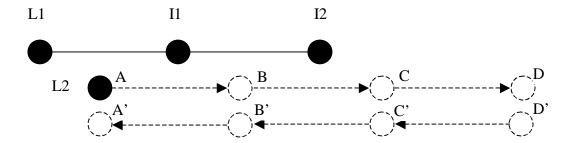
L1, I1, and I2 are located on a line. L1 can directly communicate with I1, but can not directly communicate with I2. I1 can directly communicate with both L1 and I2. Now place L2 at position A, then move L2 away and back along the dotted line  $(A \rightarrow B \rightarrow C \rightarrow D \rightarrow D' \rightarrow C' \rightarrow B' \rightarrow A')$ . During the movement, on L2 run command "ping L1 -R" to see if L2 can reach L1 and what routing path is used.
