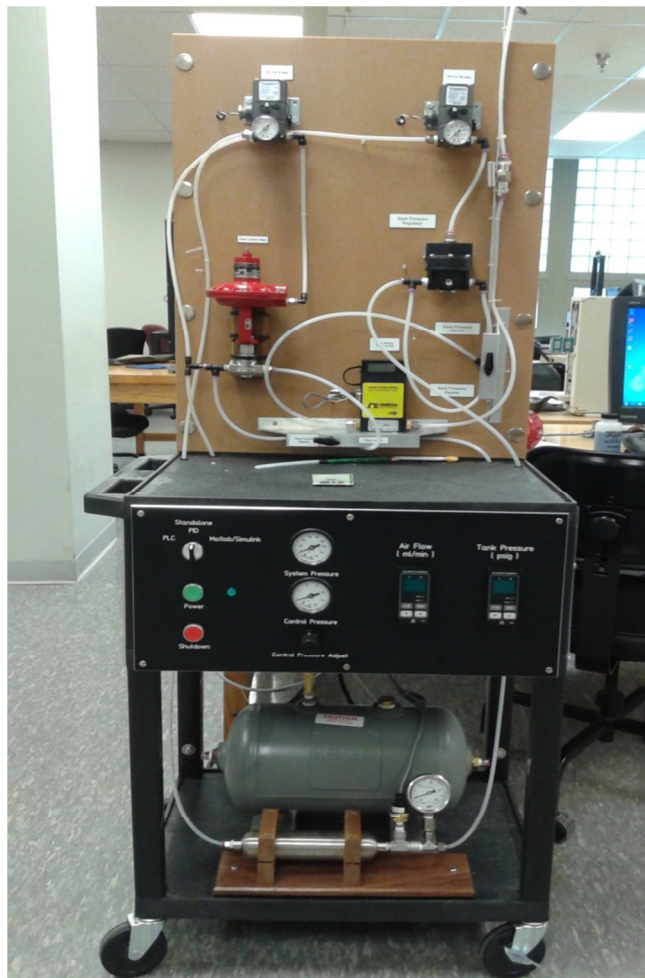
Flow Pressure Testbed
