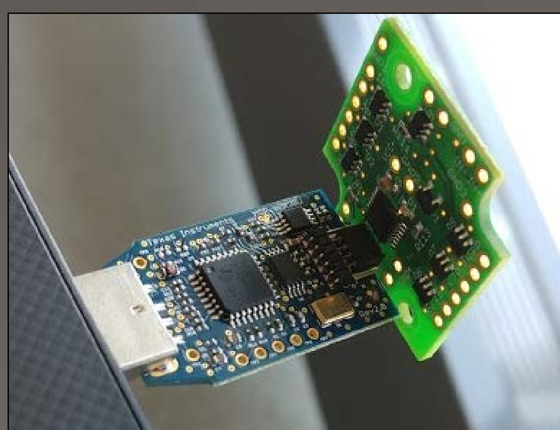
Fig 3: MSP430 Microcontroller connected to a USB Debugging Interface.
