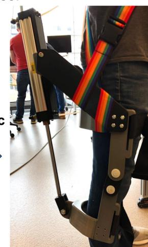
Fig 9: Pneumatic Cylinder
