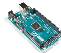
Fig 4: Arduino Mega board
