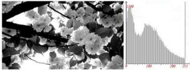
Figure 12 High contrast image and its histogram, public domain image taken from http://book.csdn.net/bookfiles/974/10097430283.shtml .
