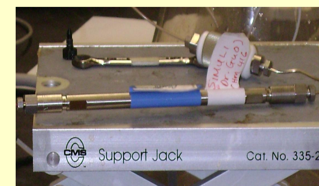
Figure 3. Atlantis T3 5 \mu m column
